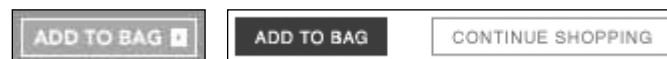
Figure 6-4. Most online stores require you to click a button to add an item to a shopping cart. This also requires a round-trip from the client to the server and a browser refresh.
